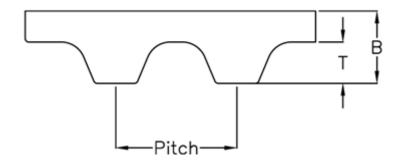
Height B mm= 2.2Height T mm= 1.2Length= 455Number of teeth= 91Pitch= 5Type= PU 20 T5 455Width= 20
